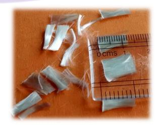
Note: Addition of fibers to a given mix may appear to decrease the slump. The workability, however, will not be affected and additional water should not be added.
